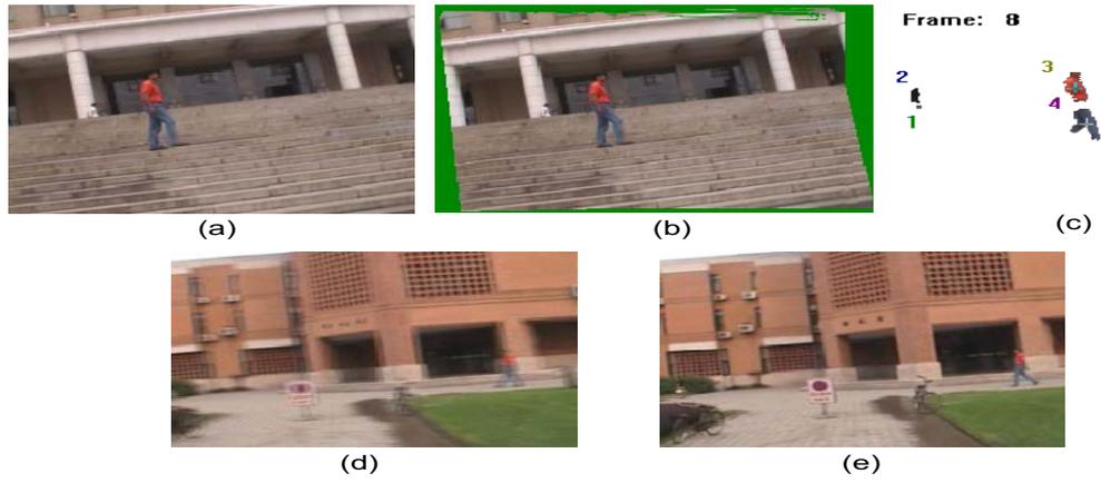
Figure 2. Hand held moving camera:(a) an image from input sequence(b) Mean background image after 8 frames (c) Foreground segmented results: Two consecutive frames taken from a moving camera (d) Camera is moving with speed(e)Camera is moving slowly
