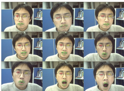
Figure 7. Some results with a web camera (results of eye contour extraction are also shown)
